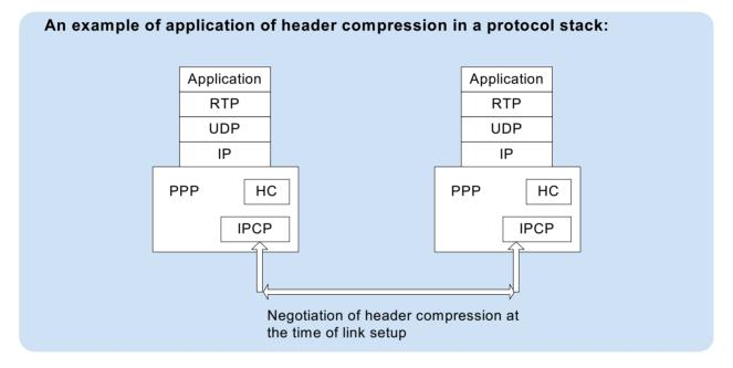
The header compression functionality must be negotiated with a set of parameters on the link. Such a negotiation protocol for ROHC over PPP has been defined in the IETF standard RFC 3241. The negotiation of the ROHC parameters like maximum context identifier, profiles supported etc takes place during link setup. The above diagram shows the location of the header compression functionality and the negotiation over a PPP link.
