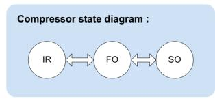
The compressor always starts in the IR state. In this state, it sends uncompressed packets to establish the context at the decompressor side. Once it gains the confidence that the decompressor has the context information, it moves to higher states of operation, either via FO state to SO state or directly to SO state. It dynamically changes its states to react to link conditions and error conditions as observed and reported by the decompressor.
