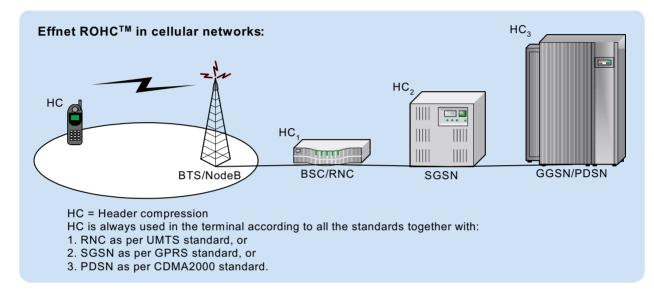
According to the 3GPP standards, the ROHC header compression function is a part of the mobile device on one end and the radio network controller (RNC) on the other end. As per the 3GPP2 standards, the ROHC header compression function is a part of the mobile device and the packet data switching node (PDSN).
