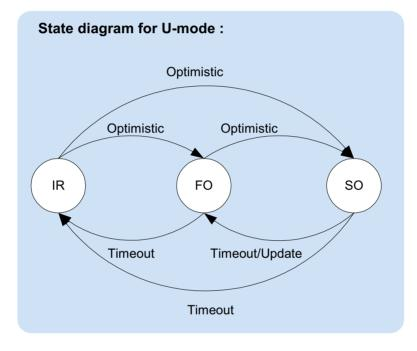
The compressor always starts in U-mode. It can move to other modes of operation if it receives a feedback (request) packet from the decompressor. As the decompressor can estimate link conditions, and knows the availability of the feedback channel, it can choose to move to other modes of operation than U-mode.
