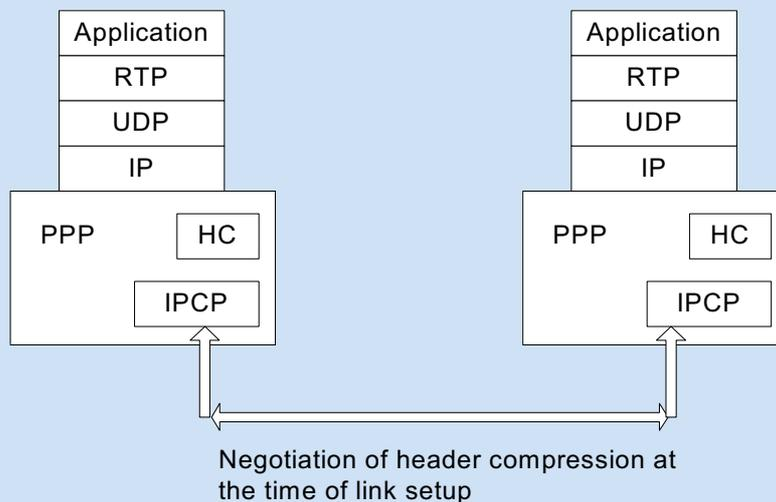
The header compression functionality must be negotiated with a set of parameters on the link. Such a negotiation protocol for ROHC over PPP has been defined in the IETF standard RFC 3241. The negotiation of the ROHC parameters like maximum context identifier, profiles supported etc takes place during link setup. The above diagram shows the location of the header compression functionality and the negotiation over a PPP link.
