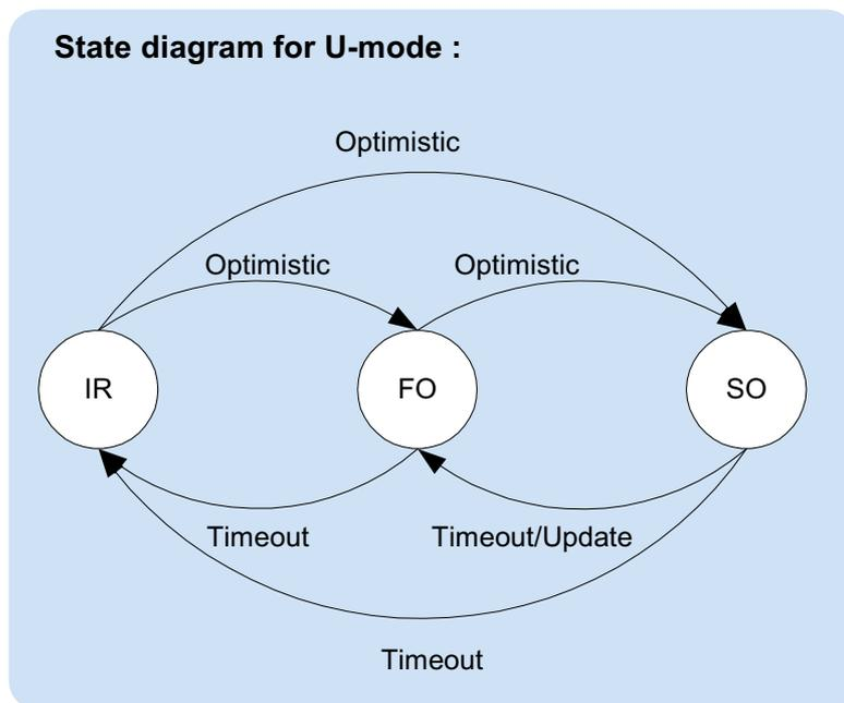
*The compressor always starts in U-mode. It can move to other modes of operation if it receives a feedback (request) packet from the decompressor. As the decompressor can estimate link conditions, and knows the availability of the feedback channel, it can choose to move to other modes of operation than U-mode.*
