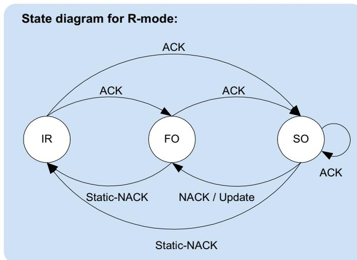
*The periodic context updating packets reduce compression efficiency compared to O-mode. R-mode tries to improve the robustness in case of packet loss and bit errors. It has very low probability of the context invalidation but if it occurs, it can result in large number of damaged packets being delivered to upper layers.*
