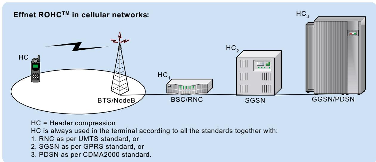
According to the 3GPP standards, the ROHC header compression function is a part of the mobile device on one end and the radio network controller (RNC) on the other end. As per the 3GPP2 standards, the ROHC header compression function is a part of the mobile device and the packet data switching node (PDSN).
