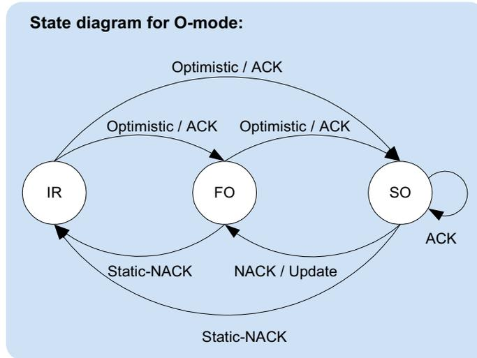
*This mode yields higher compression gains while making sparse use of the feedback channel and it reduces the packet loss due to the context invalidation.*
