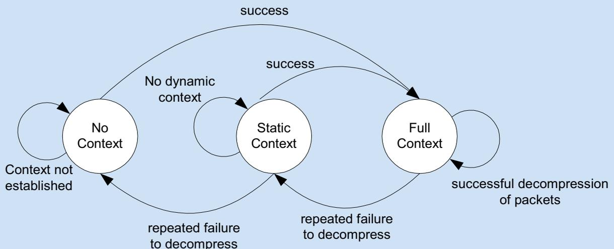
The ROHC framework defines 3 modes of operations. The selection of mode is based on parameters such as availability of feedback channel, error probabilities and header size variations. The operators of the network can choose not to use a channel to carry feedback packets for various reasons and thus limit the mode of operation of ROHC.
