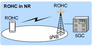
Effnet ROHCv2™ can be used in mobile broadband networks such as HSPA, LTE and NR. The standards for LTE (3GPP Rel 8+) and NR/5G (3GPP Rel15+) recommends implementation of ROHC based on RFC 5795, RFC 5225 (ROHCv2), RFC 3095 (ROHC) and RFC 4815. Effnet ROHCv2™ can also be used in cellular networks such as WCDMA. In fact, ROHC is an enabler of VoIP and provides a substantial capacity increase on all these networks.
