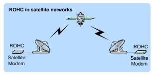
Effnet  $ROHCv2^{TM}$  also provides improved efficiency for many other network links such as satellite, WAN etc. The above examples shows how ROHC can be used on satellite or microwave links connecting multiple base-stations to BSC/RNC in a typical cellular or mobile broadband network.
