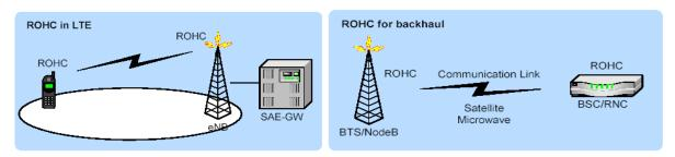
3GPP's Long Term Evolution (LTE) project focuses on enhancing the Universal Terrestrial Radio Access (UTRA) and optimizing radio access architecture. LTE has adopted packet-switch technology using end-to-end IP communication instead of traditional circuit-switching. One of the LTE specifications, Packet Data Convergence Protocol (TS 36.323) specifies use of ROHC. It supports the following ROHC framework and profiles implemented in the form of various Effnet products:
