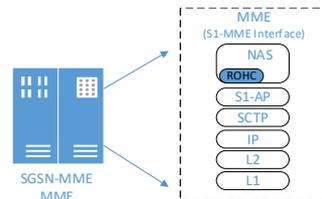
Figure 5: Integration point of ROHC in NAS in MME
