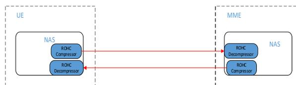
Figure 3: ROHC in uplink and downlink between UE and MME
