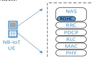
Figure 4: Integration point of ROHC in NAS in UE
