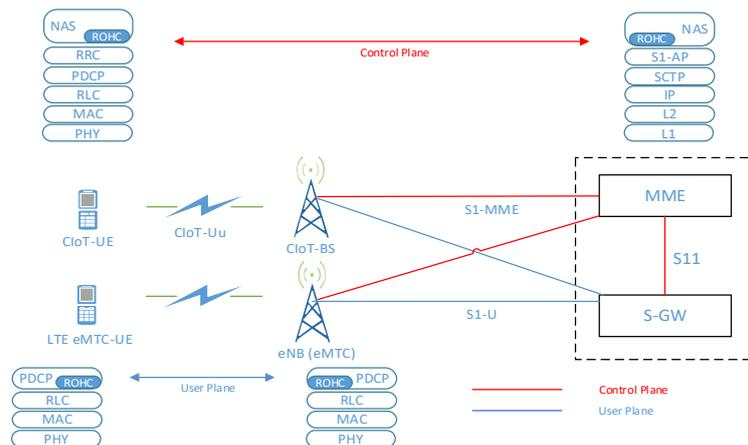
Figure 2: ROHC in control plane via NAS at UE and MME (Data over NAS Convergence Protocol) and in user plane via PDCP at UE and eNB
