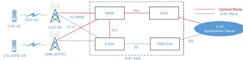
Figure 1: 3GPP Cellular IoT network architecture
