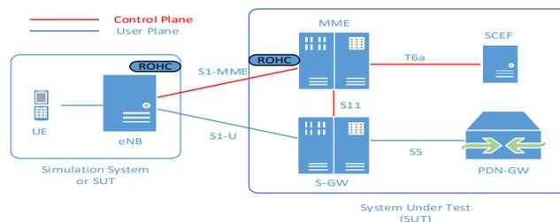
Figure 6: Integration point of ROHC in a test system and a system under test
