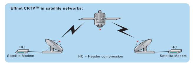
Effnet CRTP<sup>™</sup> uses the differential encoding algorithm to compress header fields and error recovery mechanisms such as header requests and TWICE. These mechanisms reduce packet loss due to bit errors and residual errors resulting in better performance and high efficiency. This header compression scheme compresses the RTP/UDP headers typically down to 2 to 4 bytes.
